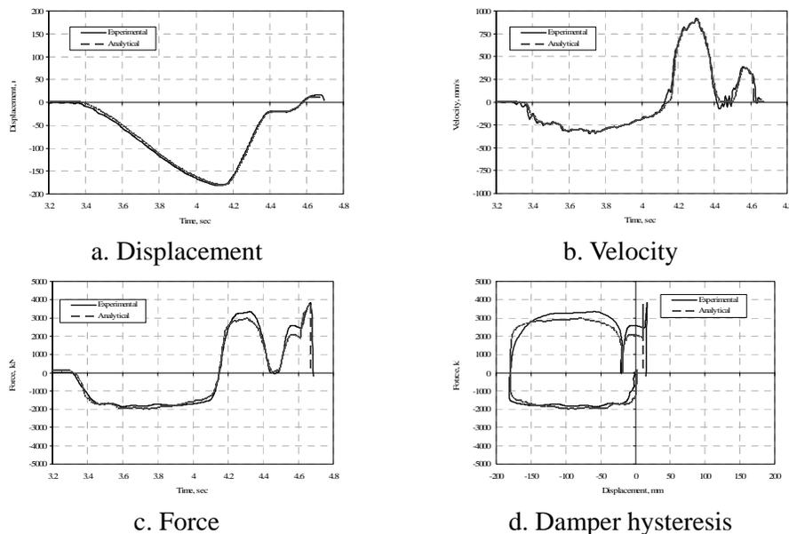
Figure 8. Experimental and analytical results
