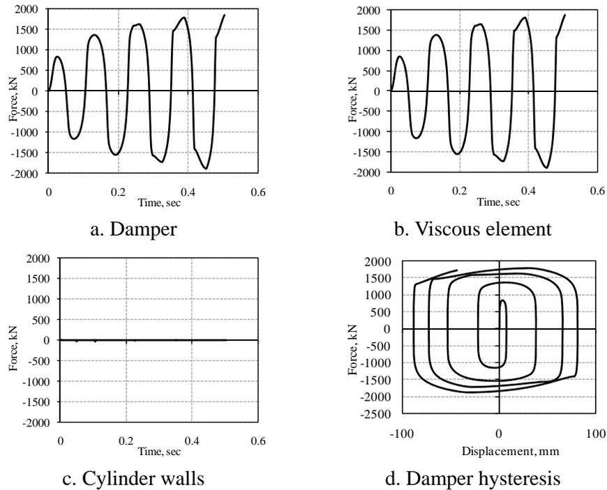
Figure 5. Response when undercut fractures
