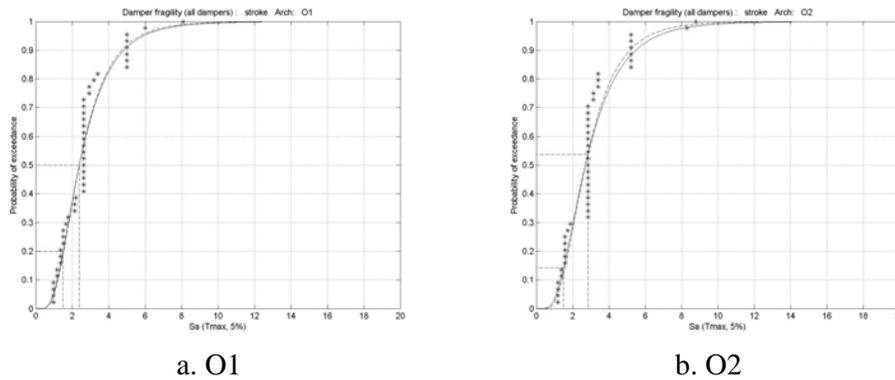
Figure 14. Damper stroke fragility
